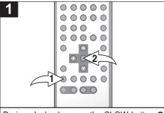
During playback, press the SLOW button 10 to move the DVD forward in slow motion speeds of 1/2, 1/4, 1/8, 1/16 and resume normal playback. The sound will be muted. You can also resume normal playback by pressing the PLAY/ENTER button 2.
